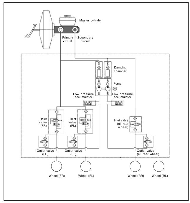
The vehicle equipped only with the ABS controls the wheel's braking force using three 3-channel 4-sensor method. The front wheels that are the primary circuit of the brake system is composed of two wheel speed sensors and two channel valves system with two inlet valves and two outlet valves. The rear wheels that are the secondary circuit of the brake system is composed of two wheel speed sensors, one inlet valve and one outlet valve. This system is similar to the one from the previous model.
