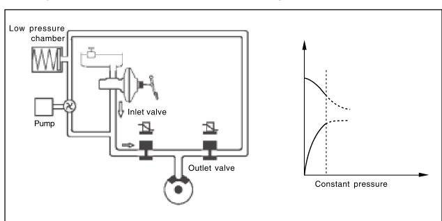
As hydraulic pressure on each wheel increases, the wheel tends to lock. In order to prevent the wheel from locking, the hydraulic valve modulator operates the inlet valve control solenoid to close the inlet valve and stop the hydraulic pressure increases. At this moment, the outlet valve is closed. This procedure helps the wheel to maintain a stable hydraulic pressure.
