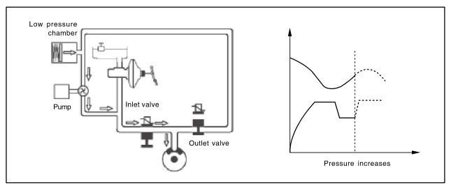
As the wheel speed increases, the inlet valve opens and the wheel's pressure increases due to the master cylinder pressure. The oil in the low pressure chamber circulates to the wheel by the pump and the wheel speed decreases as the hydraulic pressure at wheel increases. This operation continues repetitively until there are no signs that the ECU is locking the wheels. When the ABS hydraulic pressure control takes place, there may be some vibration and noises at the brake pedal.
