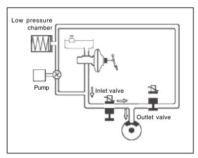
The hydraulic pressure in the master cylinder increases through vacuum booster and it is delivered to the wheel via the normal open inlet valve. At this moment, the normallyclosed outlet valve is closed. The speed of the wheel that hydraulic delivered reduces pressure is gradually.
