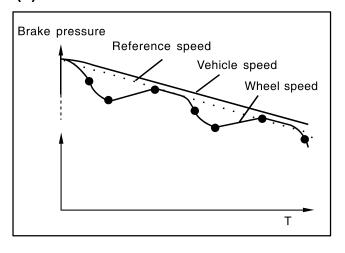
Applications of the ABS control unit The signals produced by the wheel sensors are evaluated in the electronic control unit. From the information received, the control unit must first compute the following variables:
