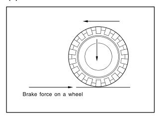
FBmax = Wheel load FR x Adhesion coefficientmh
