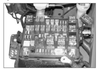
The ABS/TCS system fuse and SB2 is located at the fuse box in engine compartment.
