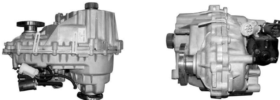
TOD system means the full time 4WD system and the registered trade mark of Borg Warner. TOD is an abbreviation of Torque On Demand.
