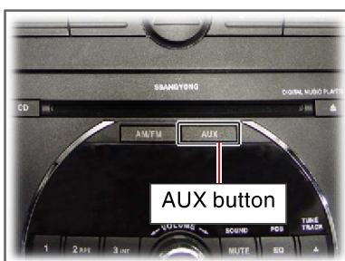
For the vehicle with common audio system, press the AUX button on upper side of the audio unit to enter the multi jack station mode. The USB mode has the higher priority than the stereo jack mode.
