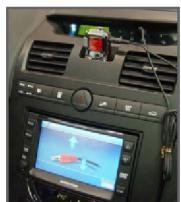
The multi jack station is an integrated unit of digital clock and various audio play devices. It also includes the stereo jack which can be connected to an external audio device and the MP3 USB jack which can be connected to the USB flash drive for playing music through the speakers on vehicle.
