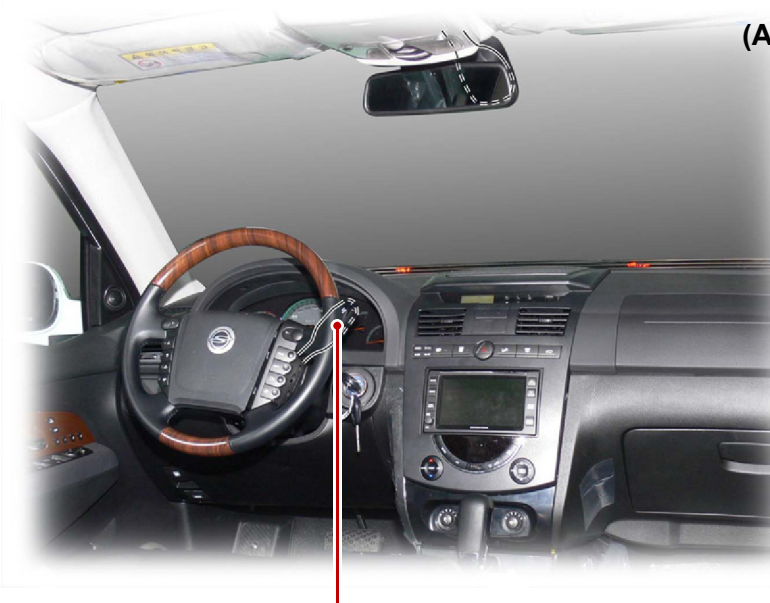
Multifunction Wiper Switch: AUTO and Sensitivity Control
