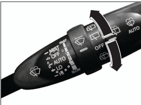
Multifunction Wiper Switch: AUTO and Sensitivity Control
