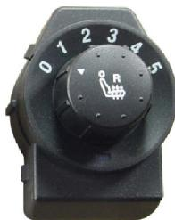
The seat warmer switch is the rotary type variable switch. The seat cushion and the seatback is heated by operating the switch and the temperature of the seat can be adjusted in five levels.
