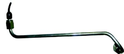
The I.D and O.D of the fuel rail between HP pump and common rail are increased according to the increased amount of fuel injection.
