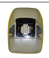
Push the front side of the button when the glass is closed then, motor actuate the operating cable to lift up the glass.
