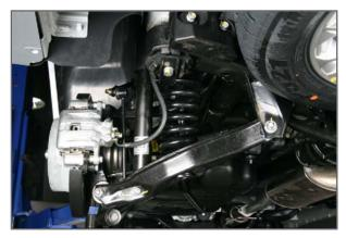
The multi-link type is used for the rear suspension to distribute the internal force (load) applied to the link while driving. Also, the change in camber or toe and shock load from the road has been minimized by optimizing the link arrangement.
