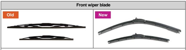
Before: Conventional type(driver: 600 mm, front passenger: 450 mm) After: Aero blade type(driver: 600 mm, front passenger: 450 mm)
