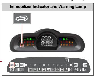
(1) When turning the ignition key to ON position, the ECU transmits the challenge message to the immobilizer unit to verify whether the key is valid. This indicator comes on when the ignition key is communicating with the engine control unit (during engine starting) and goes out after starting the engine.
