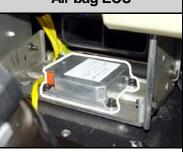
Sends the vehicle collision signals to STICS.
