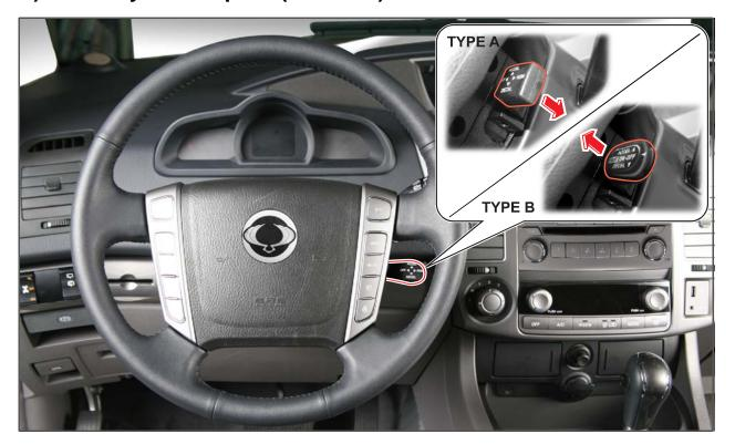
Even if the cruise control is cancelled, the previous set cruise speed can be recovered by pushing (Type A) or pulling (Type B) toward the cruise control lever when the current vehicle speed is over 36 km/h without an acceleration intervention. But if you turn off the ignition switch, the memorized set speed is cleared and you cannot recover the previous set speed.
