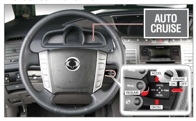
The cruise control is an automatic speed control system that maintains a desired driving speed without using the accelerator pedal.
