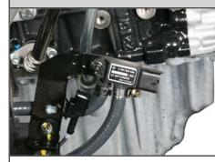
Measures the difference between inlet and outlet pressures of CDPF.
